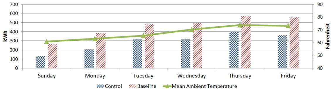
Fig. 6. Daily energy consumption of MOBS and baseline controllers and daily mean ambient temperature.
