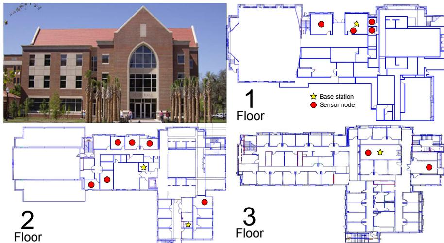
Fig. 1. Pugh Hall and the locations of the wireless nodes (circles) on each floor. Base stations are represented by stars.
