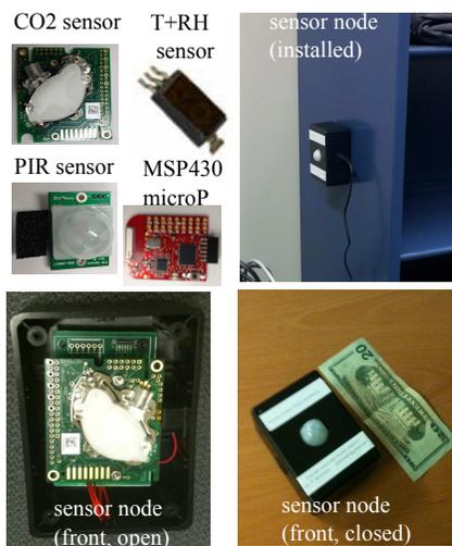
Fig. 2. Wireless sensor node deployed in Pugh Hall [14].
