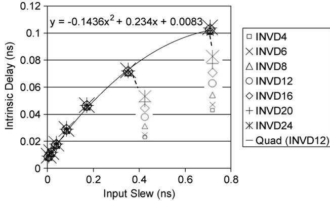
Fig. 1. Dependence of repeater intrinsic delay on input slew and inverter size. Intrinsic delay is essentially independent of repeater size and depends quadratically on input slew.
