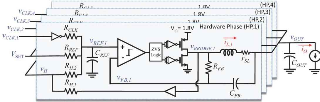
Fig. 3. Diagram of the proposed nonlinear, unlatched PWM control scheme.
