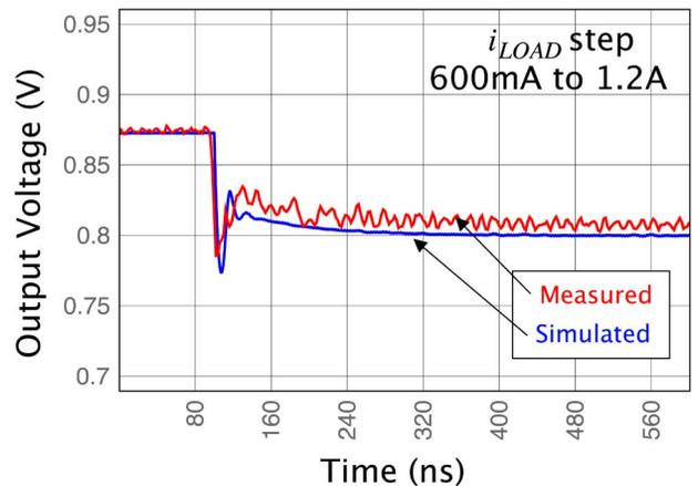
Fig. 10. Measured and simulated load-current transient step response.
