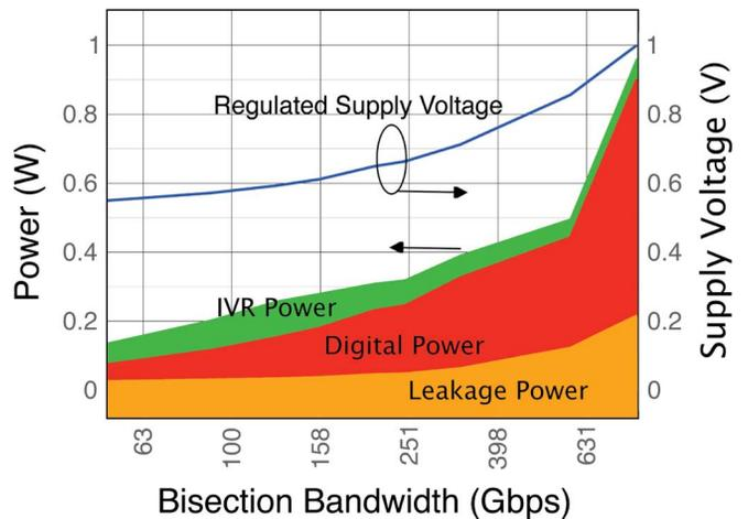
Fig. 13. NoC power consumption as a function of bandwidth (operating frequency).
