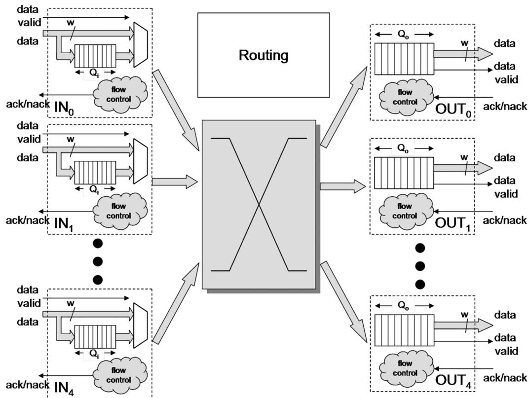
Fig. 15. Network-on-chip router micro-architecture.
