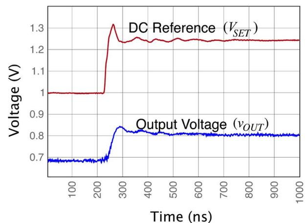
Fig. 11. Measured input step-up response.
