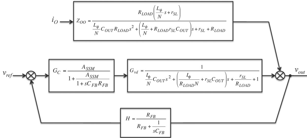
Fig. 6. Small-signal model of control loop.
