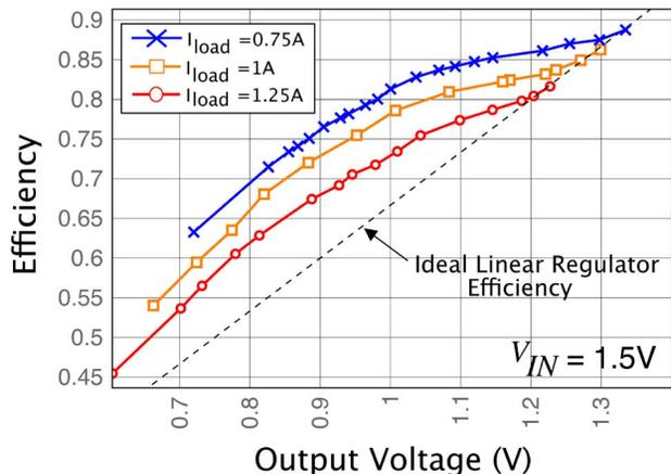
Fig. 12. IVR efficiency as a function of output voltage,  $v_{OUT}$ .
