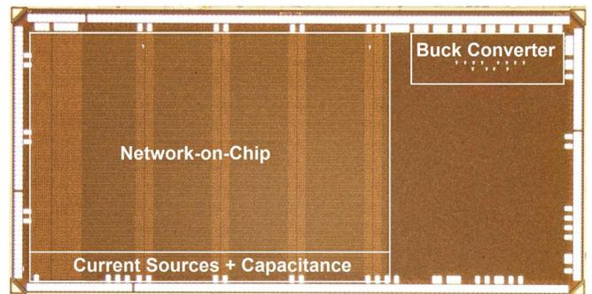
Fig. 8. Photo of test chip.
