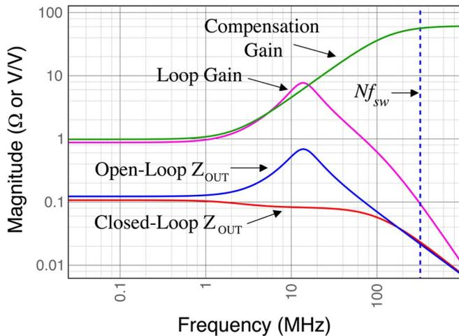
Fig. 7. Small signal transfer functions and output impedance of proposed control scheme.
